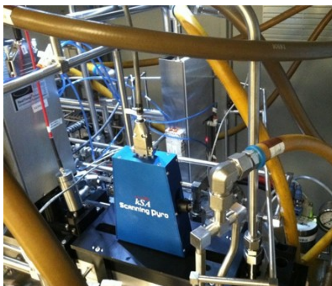
Mechanical drawing of the kSA SPYRO-465 footprint and a photograph of the kSA SPYRO-465 on a k465i reactor.
