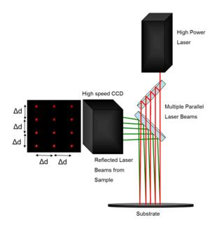
The kSA MOS also features the patented and automated servo-motor control of an optical flat mirror to provide fully automated tracking capability during data acquisition. This feature is of particular use in monitoring curvature/stress during high temperature annealing where thermal expansion may cause angular displacement of the sample and thus the reflected laser array.
